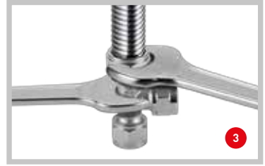
Assembly of T piece with two tools.
